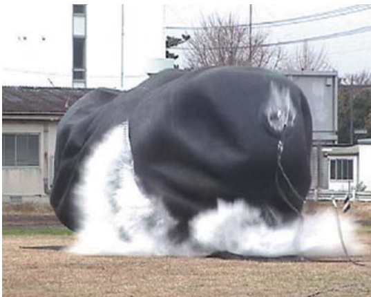
Fig.3.2 Burst Test at 0% Deflection
