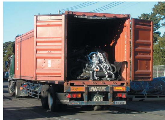
Fig.11-2 \phi 3300 \times 6500\text{L-P80} Transportation by Open-top Container
