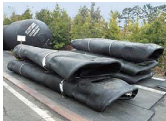
Fig.11-4 \phi 3300 \times 6500\text{L-P50} Body Only under the deflated condition
