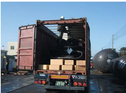
Fig.11-3 \phi 2500 \times 5500\text{L-P50} Transportation by Open-top Container
