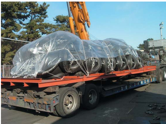
Fig.11-1 \phi 4500 \times 9000\text{L-P80} Transportation on Steel Pallet
