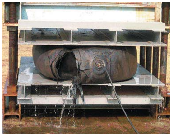
Fig.3.3 Burst Test at 60% Deflection
